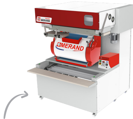
Compact Page semi-automatic group: Intermediate proofer + Incorporated moulder.
